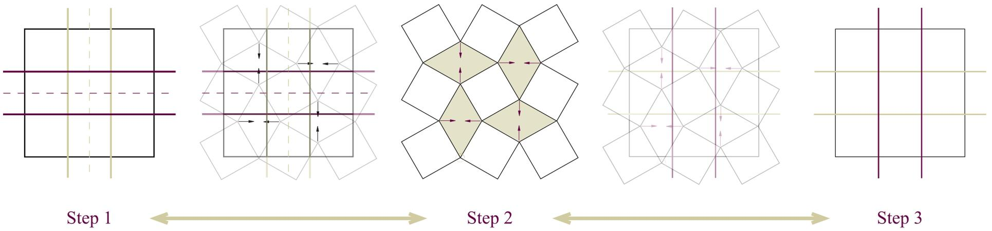
THIS DIAGRAM SHOWS THE PROCESS IN WHICH THE PRISMS ROTATE IN HARMONY. CONNECTING EACH PRISM TO ITS PARTNER EDGE IS CRUCIAL. THE EDGES MUST BE CONNECTED IN OPPOSITION IN ORDER FOR THE ROTATE TO OCCUR. THIS CONNECTION ALLOWS FOR ONE TO MOVE ONLY A SINGLE PRISM TO ALLOW ALL THE PRISMS TO MOVE. THE COLOR FILL IN "STEP 2" REPRESENTS THE VOIDS THAT LIGHT SHINES. THE SHAPE OF THE VOIDS DEPENDS ON THE ANGLE OF THE ROTATION IN THE SYSTEM.
