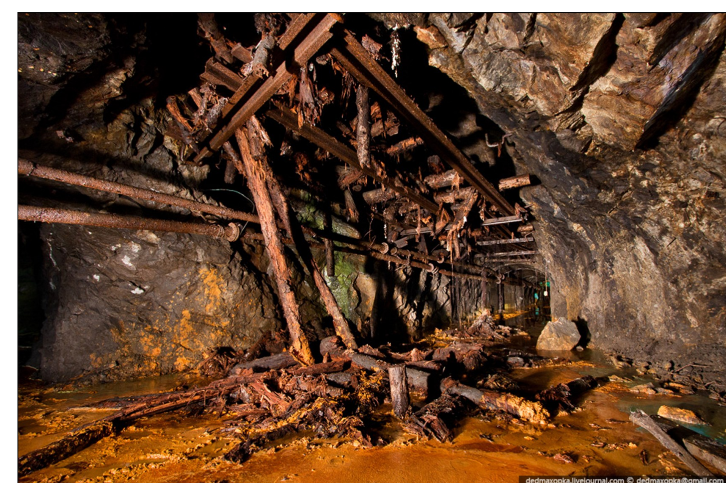
Figure 1: An abandoned mine with visible Fe dissolution orange and green
